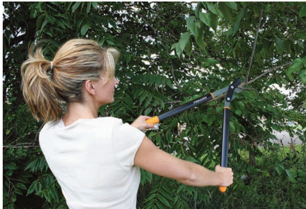
The gear or lever mechanisms on this lopper increase leverage and maximize cutting power. (Photos: Fiskars Garden & Outdoor Living)
